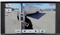
Utilizes 3 cameras to provide multiple views along with steering guidance graphics to assist in backing and maneuvering a trailer
