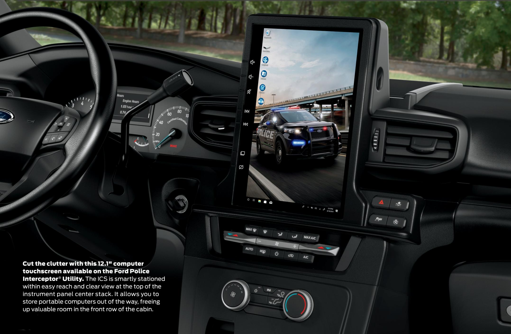
**Cut the clutter with this 12.1" computer touchscreen available on the Ford Police Interceptor® Utility.** The ICS is smartly stationed within easy reach and clear view at the top of the instrument panel center stack. It allows you to store portable computers out of the way, freeing up valuable room in the front row of the cabin.
