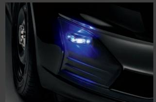
Side warning light housing. Features integrated, custom-designed LED prep assembly. Shown with LED lights (driver side red; passenger side blue) – included with Front Headlamp Lighting Solution (14A).
