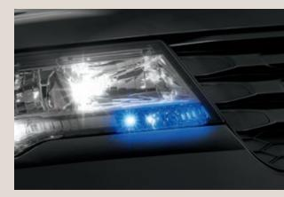
Forward indicator pocket warning lamps. Custom-designed, multifunctional Park/Turn/Warn (PTW) LED assemblies integrated into the headlamp system.
