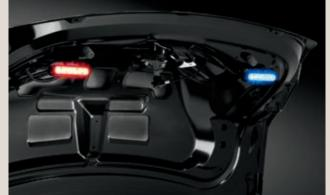
**Police back-window lights.** Includes (2) backlit flashing, linear high-intensity LED lights (driver side red; passenger side blue) with surround cover mounted inside the back window glass. **Police trunk lights.** Includes (2) backlit flashing, linear high-intensity LED lights (driver side red; passenger side blue) mounted inside the decklid; lights activate when trunk is open.
