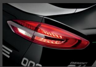
**Police taillamp.** Includes base LED lights with wig-wag module functionality with alternating reverse lights and taillamp lights only.
