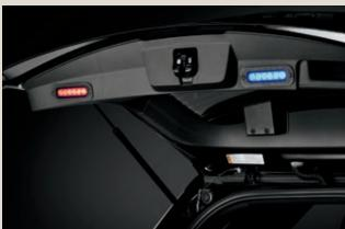
**Police liftgate-glass lights.** Includes (2) backlit flashing, linear high-intensity LED lights (driver side red; passenger side blue) with surround cover mounted inside the liftgate glass. **Police liftgate lights.** Features (2) backlit flashing, linear high-intensity LED lights (driver side red; passenger side blue) mounted inside the liftgate lip; lights activate when liftgate is open.
