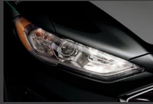
**Police headlamp.** Includes base headlamp with high-beam wig-wag function plus (2) LED side warning lights (driver side red; passenger side blue).
