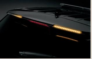
**Rear spoiler traffic warning lights.** Includes (2) backlit flashing, linear high-intensity LED lights (driver side red; passenger side blue) mounted on the edge of the rear spoiler. Lights can be programmed for tricolor (red, blue, amber) patterns; also features amber-only traffic direction mode.
