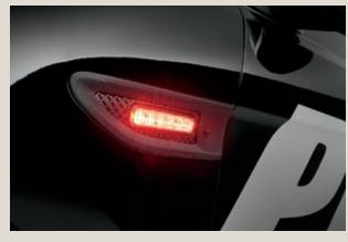
Police side lamps. Fender side markers feature backlit flashing, linear high-intensity LED lamps.
